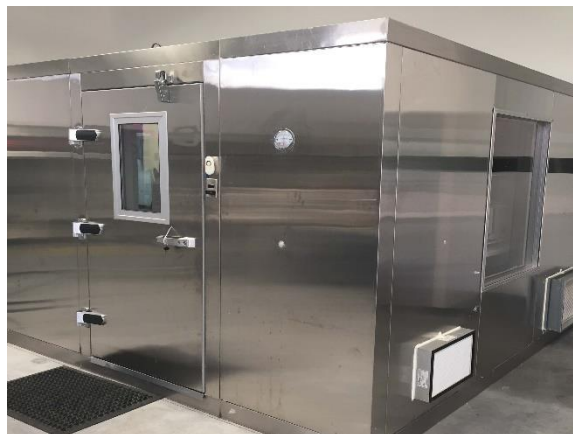
Figure 2: The 30 m 3 bioaerosol testing chamber at ARE Labs adheres to AHAM AC-5 standards and ASHRAE 241 criteria. The chamber is equipped with HEPA filtered air in/out, multiple bio aerosol sampling ports, decontamination, and pressure balance.
